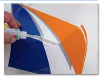
At this point if you have any areas where excess glue has run along the cover-ing, you can remove it with some acetone on a paper towel. Acetone will not hurt iron-on covering (if you covered it with something other than an iron-on covering, or if the area is painted, skip the acetone). After a few hours, you may see a white film around the gluing area. Again, a little acetone will wipe this right off.
