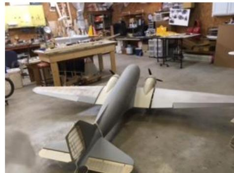
led lights for the wing and tail navigation lights, and 2 Cree 1 inch 1300 lumen for the landing lights. The landing lights are controlled using a Rexel ignition kill switch mixed with the flap channel. The aircraft also features a side door that is controlled by a servo via a switch on the transmitter. The overall aircraft weight came out to be around 57 lbs. I will be heading to the Fredericksburg RC club in mid May to test fly and obtain the AMA Large model aircraft documentation.
